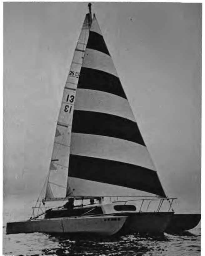
In light airs, the cutter's huge genoa (above) provides enough area to glide along on a zephyr. The forestay and runners are released for easy tacking.
