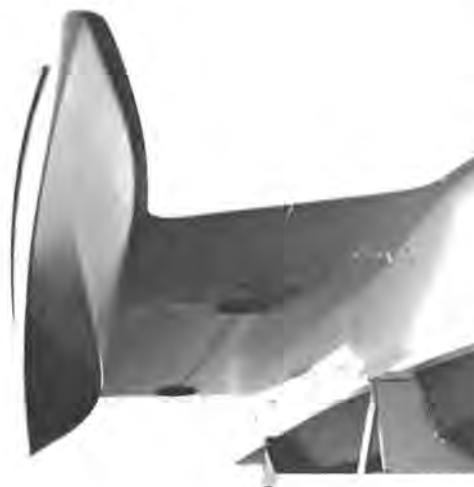
CARAVEL's floats were extremely asymmetric, with flat bottoms. Note wide hull spacing.
