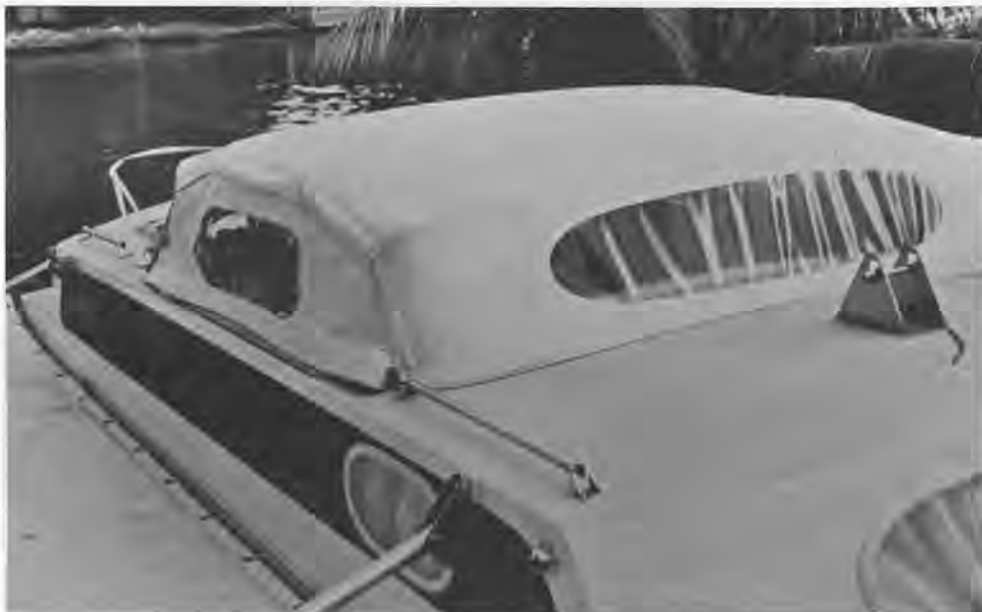
The central cockpit is ideal for covering with several types of "dodgers" or "boomtents". Some of these can be used under sail; others expand the accommodations for harbor-living by making the cockpit into the social center of the boat; another separate cabin.
